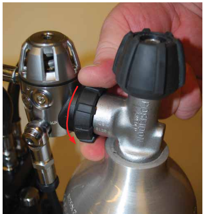
Figure 1-47. Hand tighten the diluent swivel nut.
