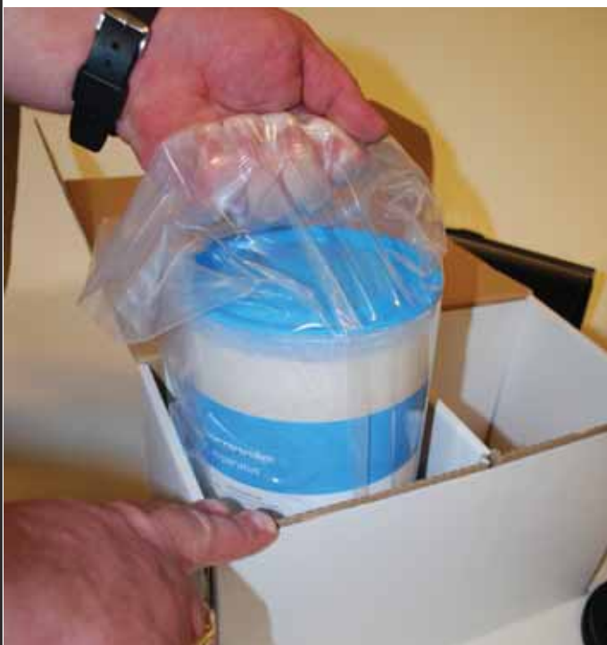
Figure 1-20. Unpacking a fresh SofnoDive 797 CO 2 absorbent cartridge.
