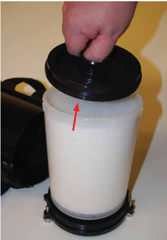
Figure 1-16. Remove the cartridge top plate.
