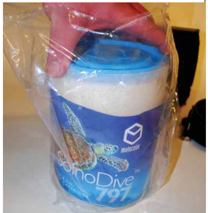
Figure 1-21. Opening the sealed SofnoDive 797 air-tight shipping envelope
