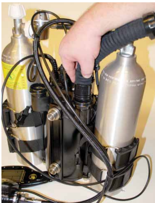
Figure 1-53. Insert the rear left hose into the gas processor housing.
