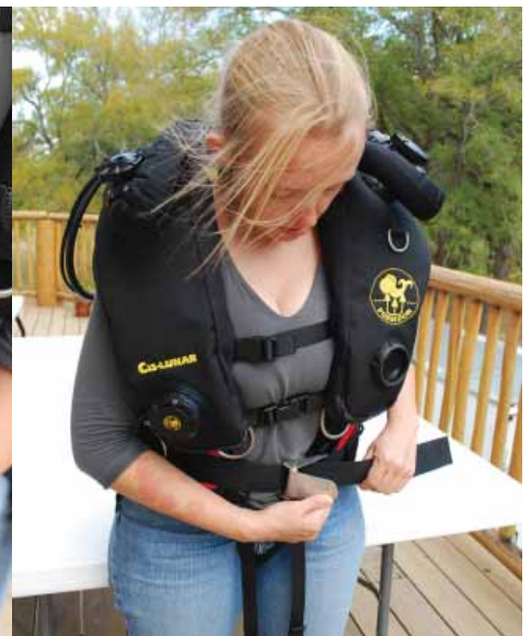
Figure 1-100. Attach the backpack harness main waist buckle and cinch tight.
