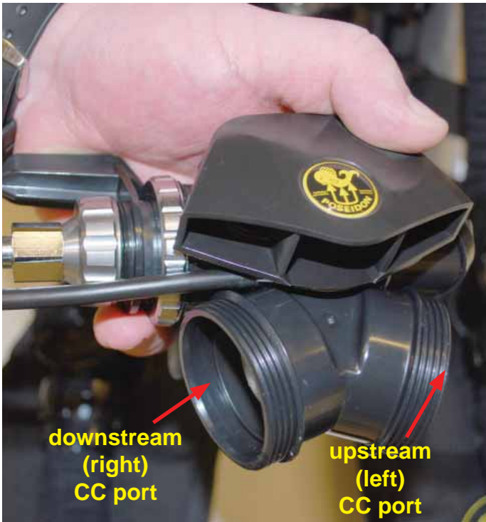
Figure 1-70. Mouthpiece closed-circuit (CC) inhalation and exhalation port definitions.
