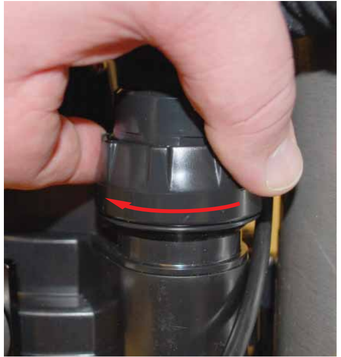
Figure 1-56. Hand tighten the swivel capture nut: Do NOT use tools or over-tighten.
