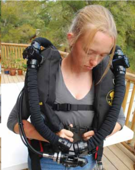
Figure 1-96. Attach the counterlung cross strap.
