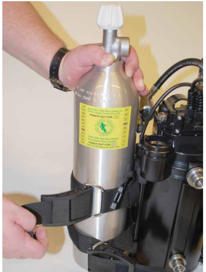
Figure 1-39. Pull the strap tight through the cam buckle.
