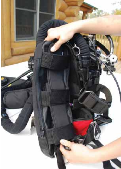
Figure 1-90. Attach the bottom velcro retainer to the left harness strap.
