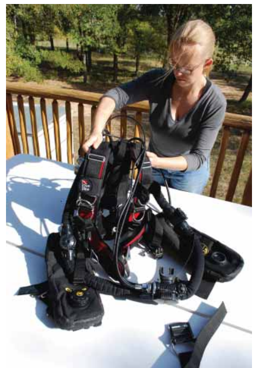
Figure 1-82. Insert the cam band such that the rig rides at the right height.
