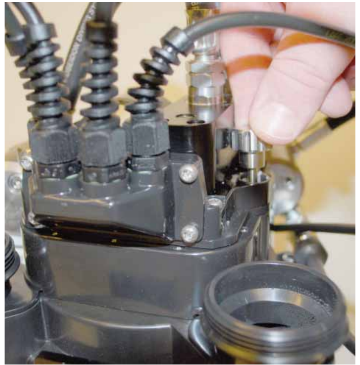
Figure 1-34. Firmly screw down the hand nut on the left side of the electronics housing (use NO tools)
