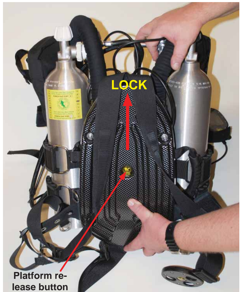
Figure 1-77. Push the Platform upward to lock.
