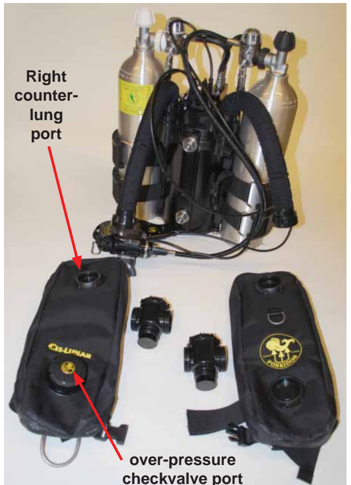
Figure 1-58. Lay out both left and right hand counterlungs and their water diversion manifolds.
