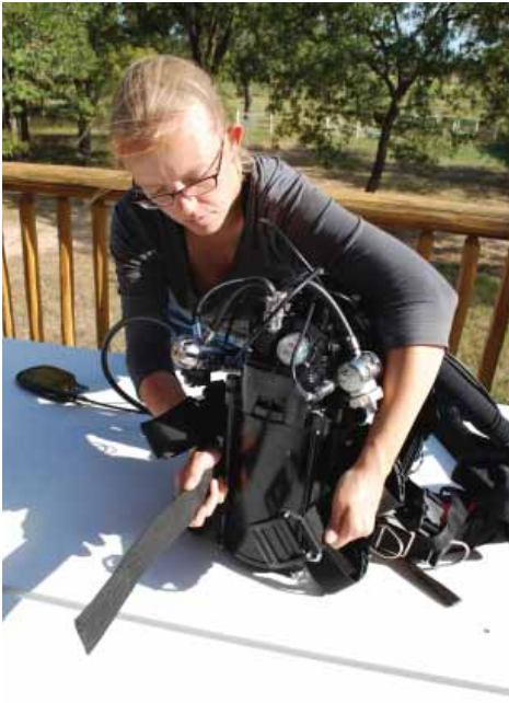
Figure 1-83. Pass the cam band around the center of the gas processor.
