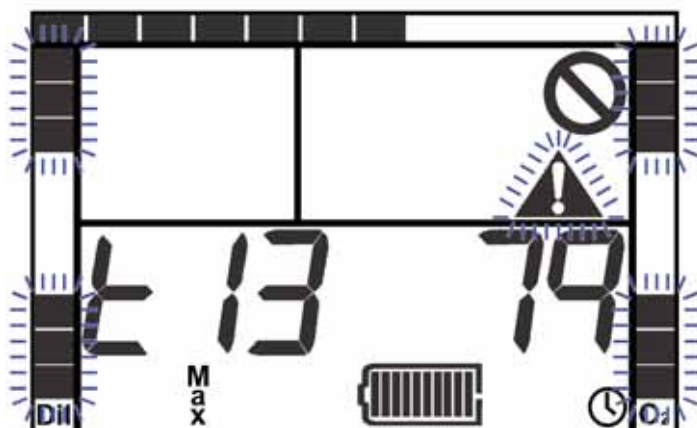
Figure 2-4. Test 13 (Backlight Power consumption), displaying test number on the left and remaining time (in approximately 0.1 -second increments) on the right.
