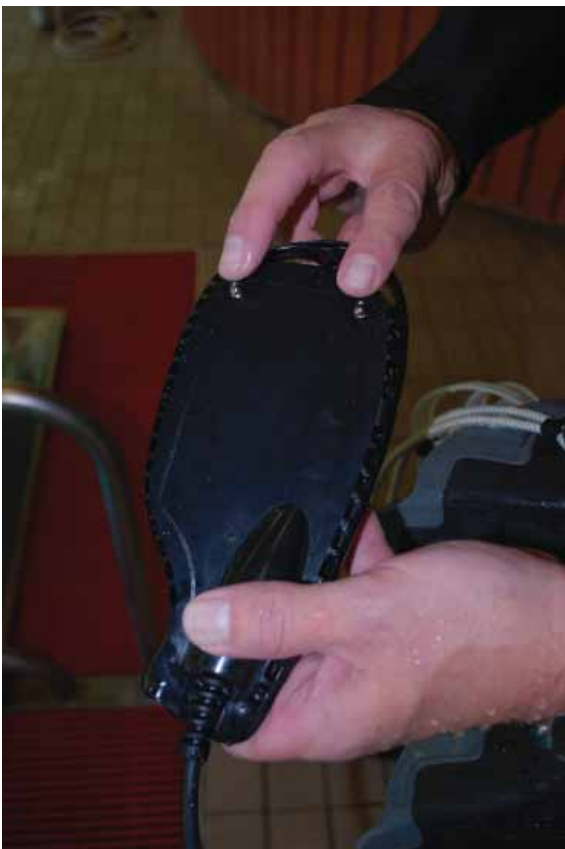
Figure 2-1. Connect the wet switch on the back of the Primary Display for Power-Up.
