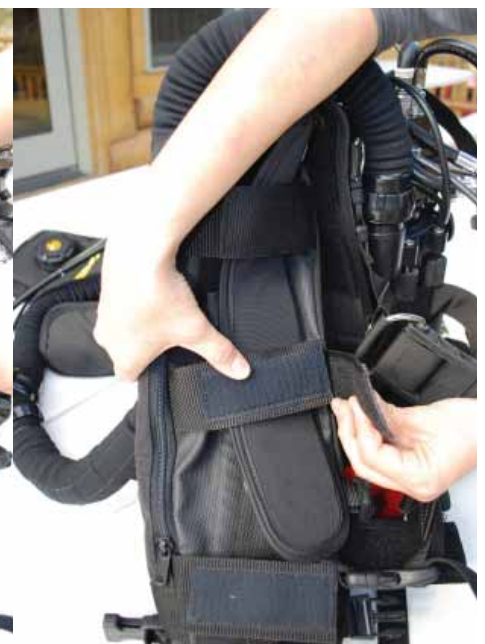
Figure 1-90. Attach the middle velcro retainer to the left harness strap.
