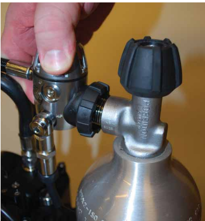
Figure 1-46. Align the diluent regulator with the diluent cylinder female DIN thread.
