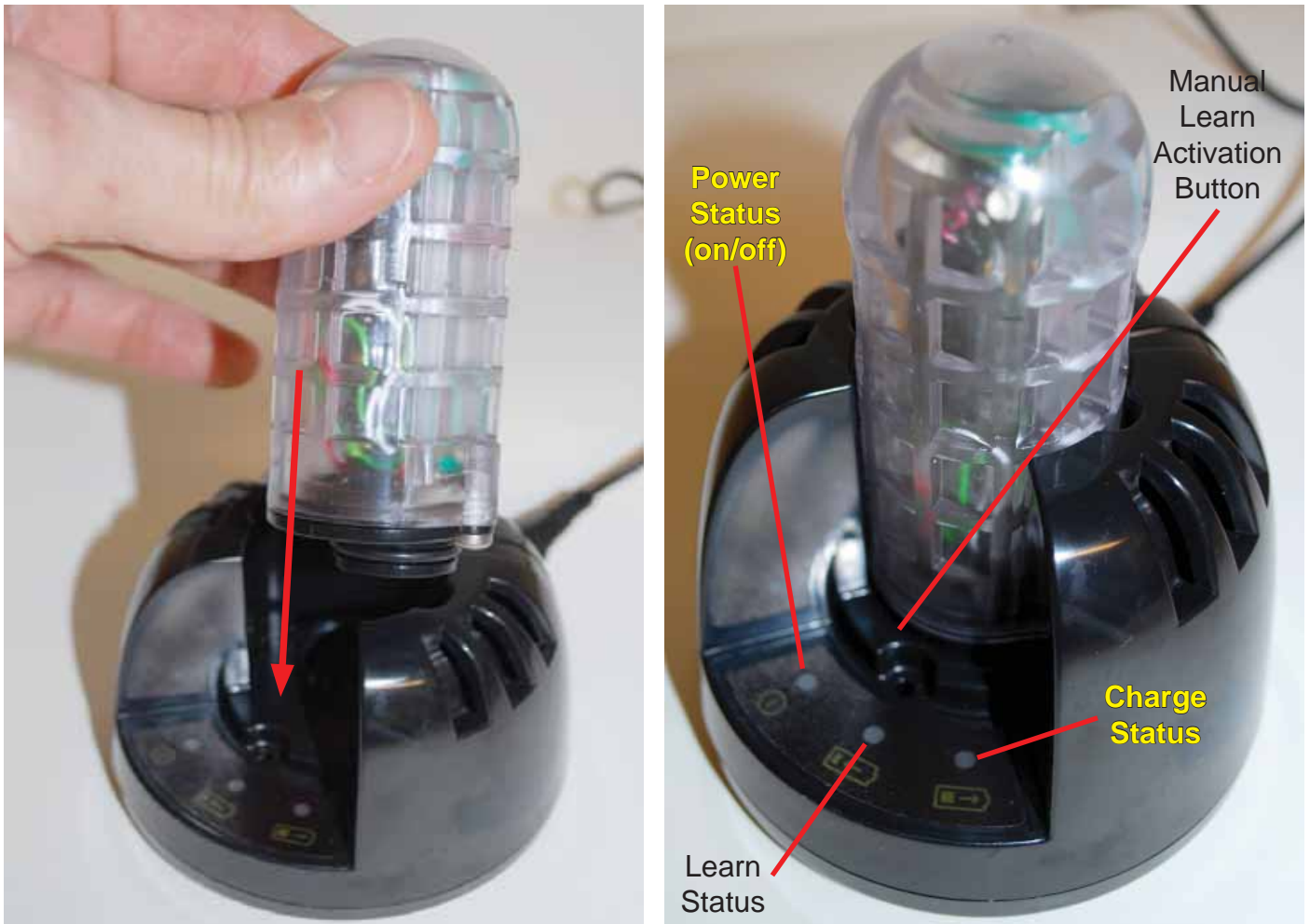
Figure 1-8. (Left): Inserting the smart battery into the desktop charging station. The battery screw posts align with the vertical slots; the battery is pushed down until the contact post mates with the offset cylindrical receiver hole. (Right) the battery properly inserted into the charger. See the text for definitions of the status indicator lights.
