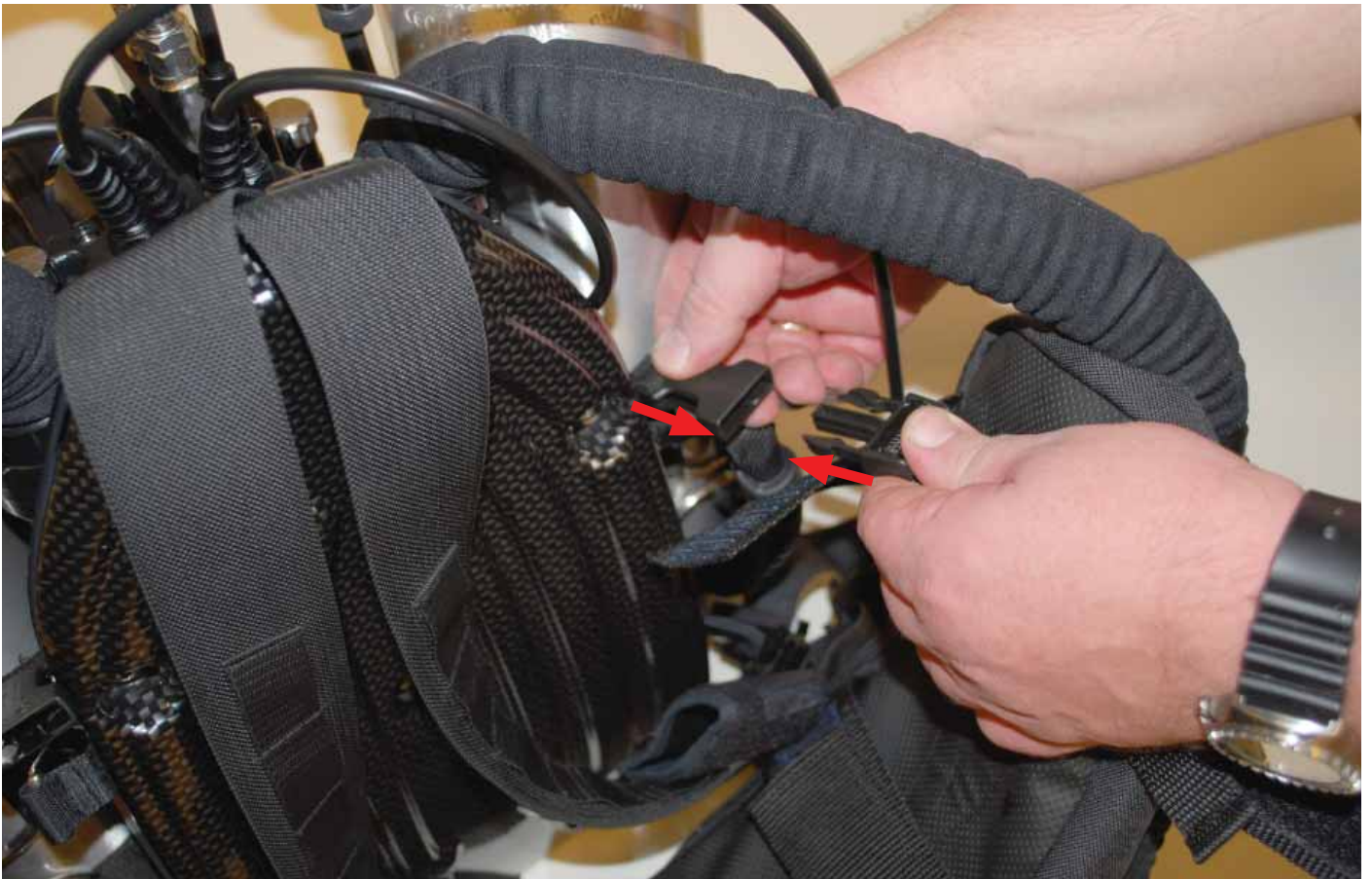
Figure 1-78. Fasten the upper counterlung position with the adjustable-length quick-connect buckle.
