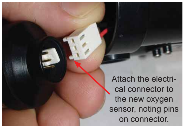
Figure 4-6. Attach the electrical connection to the sensor.
