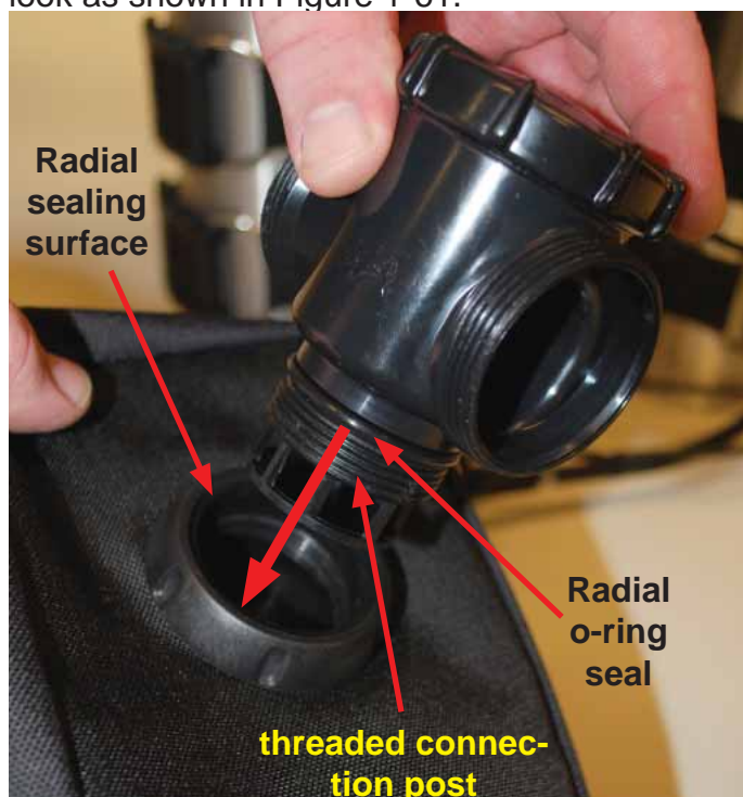
Figure 1-60. Insert the right hand water diversion manifold into the port on the right counterlung.
