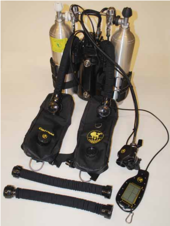
Figure 1-66. Lay out the two front breathing hoses.
