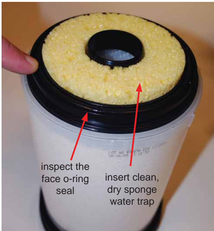
Figure 1-24. Insert cartridge top plate and sponge water trap, final inspection of face seal o-ring
