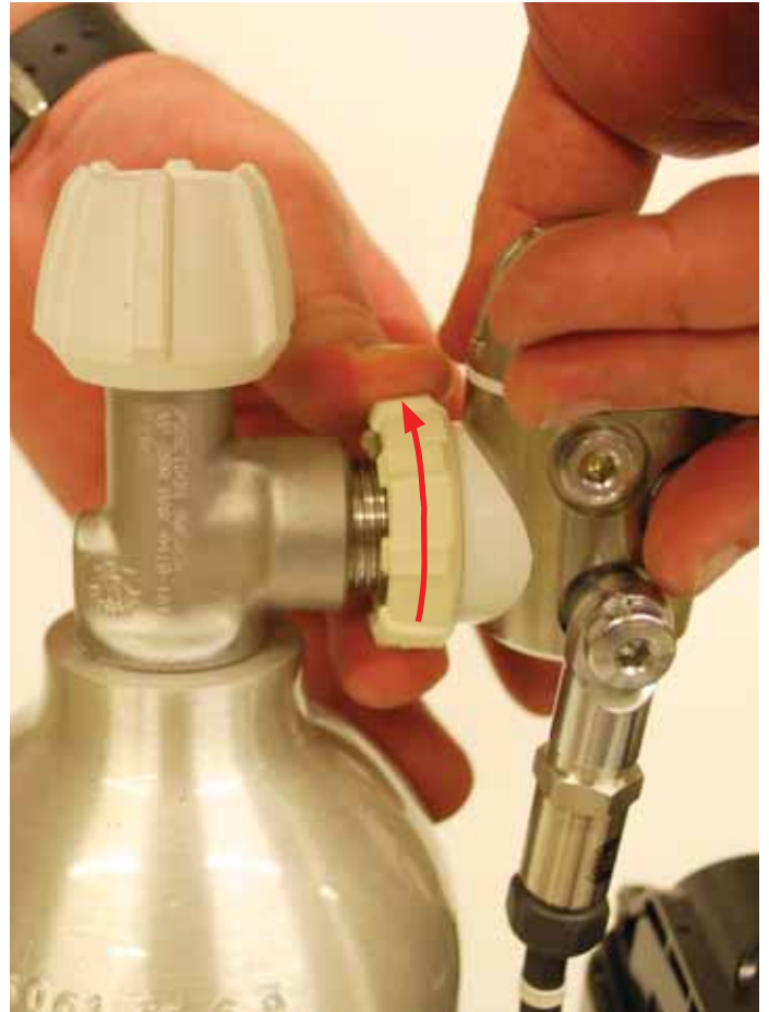
Figure 1-43. Hand tighten the oxygen swivel nut.
