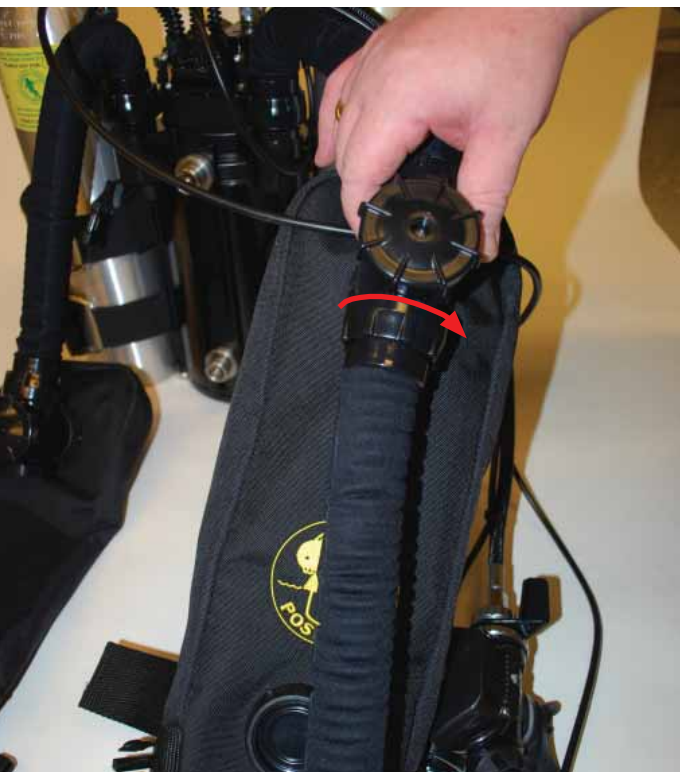
Figure 1-68. Hand tighten (clockwise) the swivel nut for the left front breathing hose at the left front shoulder port. DO NOT use tools or over-tighten.
