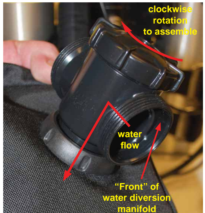
Figure 1-61. Clockwise tighten the water diversion manifold into the right counterlung shoulder port.
