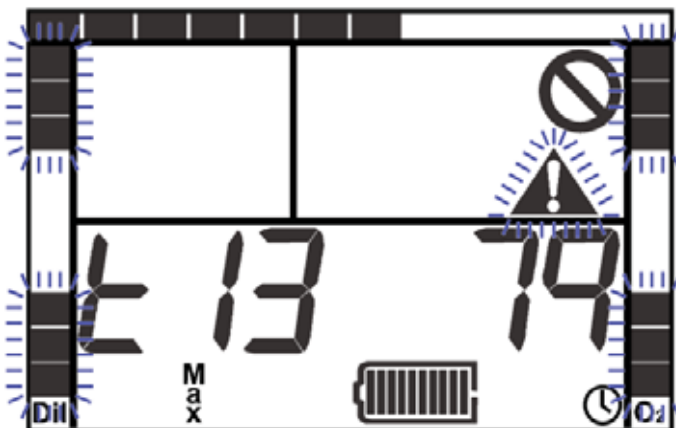
Figure A1-1: Test 13 (Backlight Power consumption), displaying test number on the left and remaining time (in approximately 0.1 -second increments) on the right.
