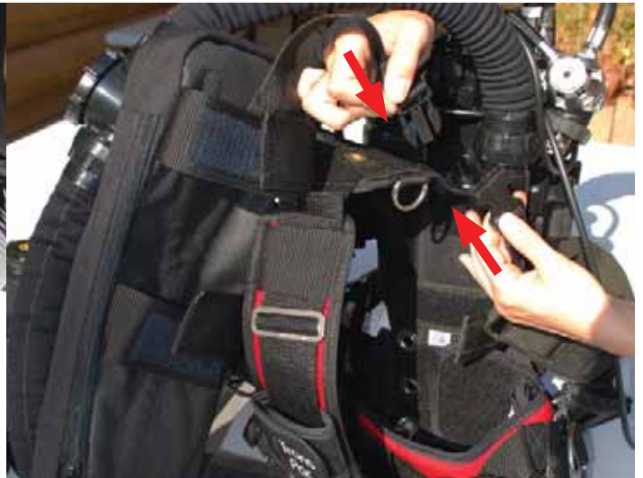
Figure 1-87. Attach the left counterlung upper positioning buckle.
