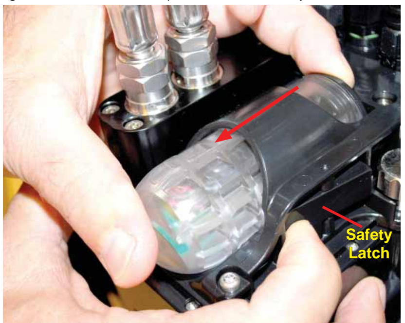
Figure 1-7. Removing the Smart Battery.
