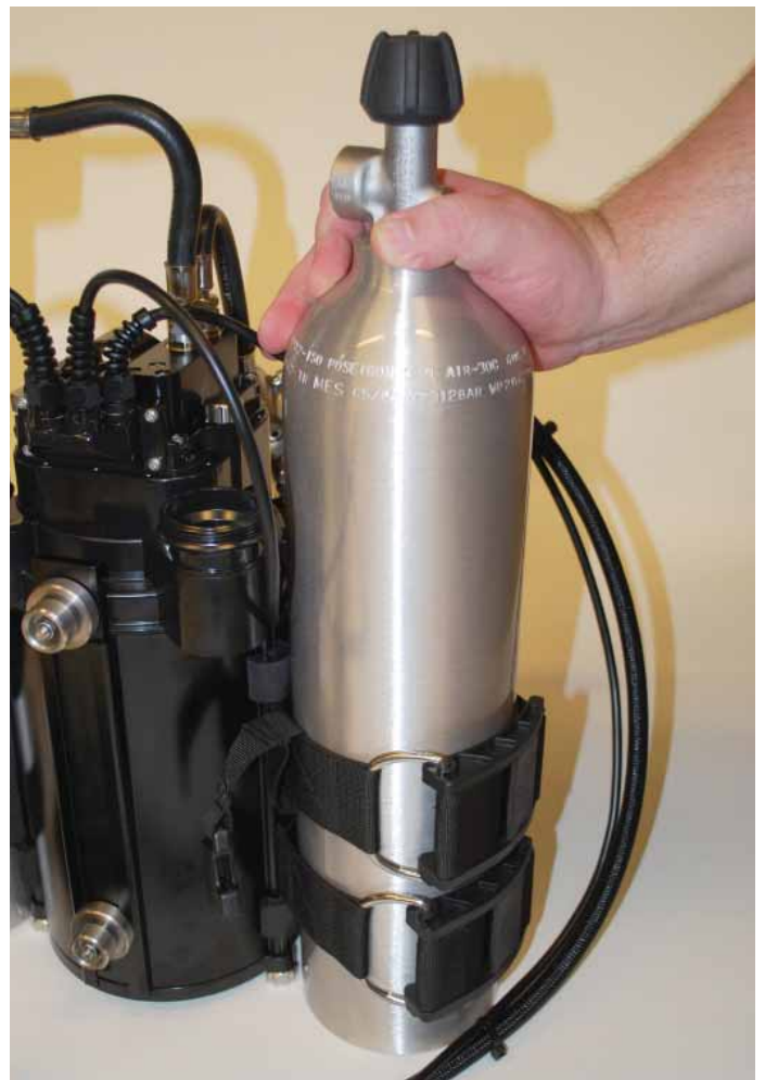
Figure 1-45. Follow the same procedures of steps 36-39 to tighten and latch the diluent cylinder bands.
