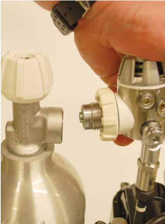
Figure 1-42. Align the oxygen regulator with the oxygen cylinder female DIN thread.
