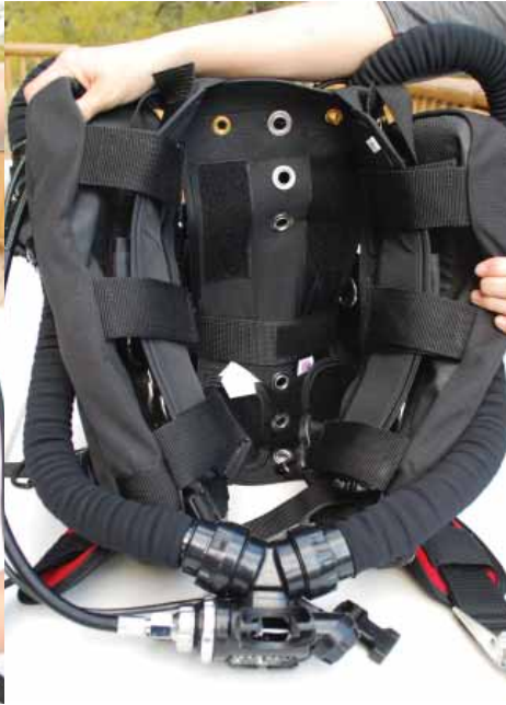
Figure 1-91. Repeat the procedure for the right counterlung & harness strap.
