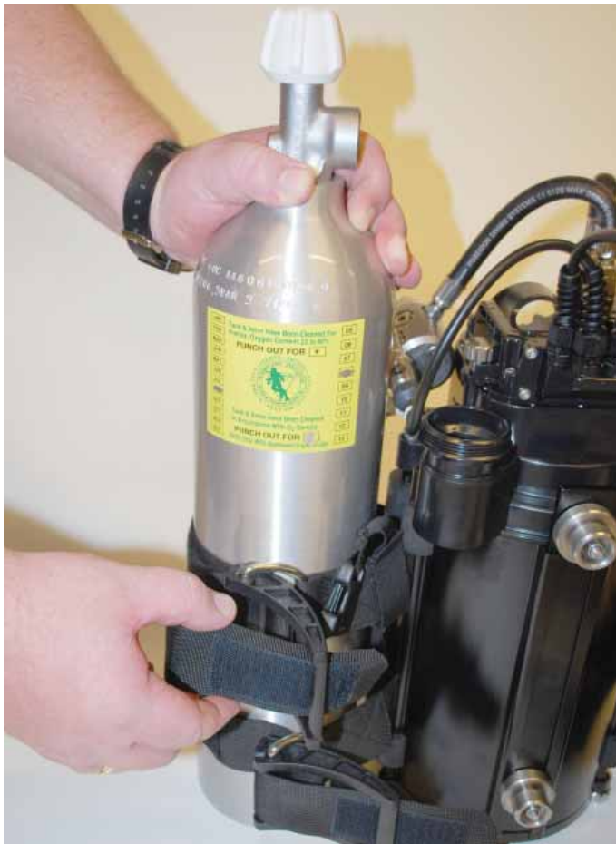
Figure 1-38. Thread the strap through the cam buckle.
