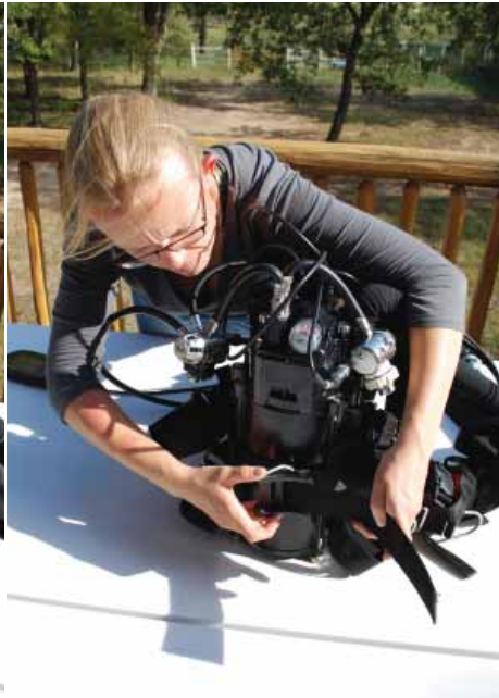
Figure 1-84. Thread the cam band as for a normal Scuba cylinder.
