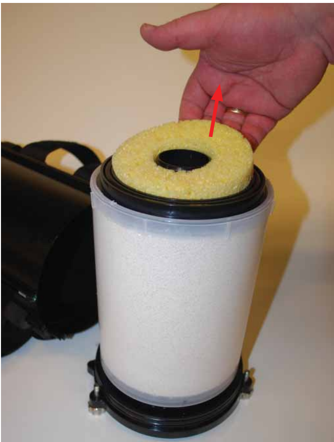
Figure 1-14. Lift and remove the upper sponge.
