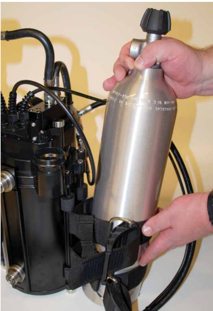
Figure 1-44. Insert the diluent cylinder into the two right cam straps.
