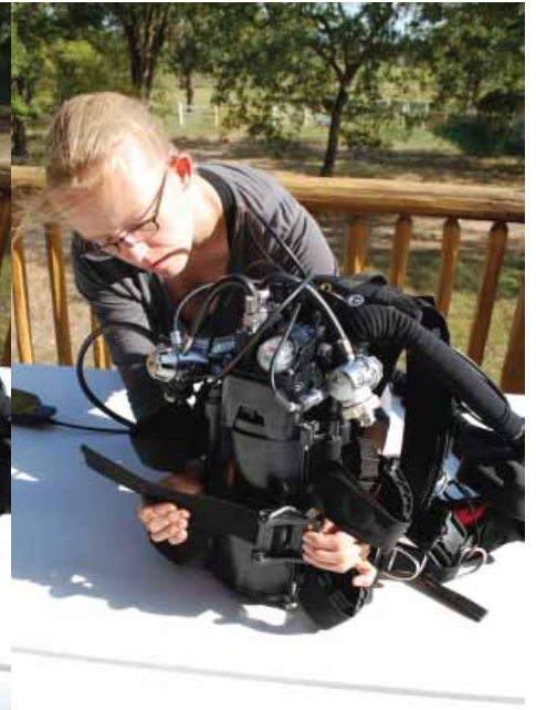
Figure 1-85. Snug the cam band at the mid height of the gas processor.
