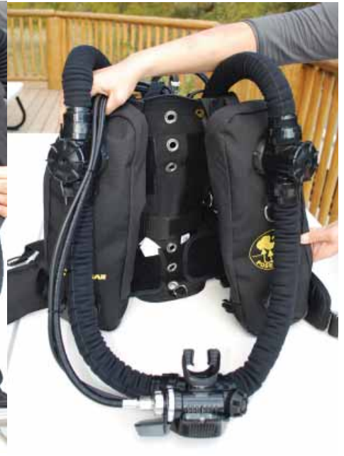
Figure 1-93. Adjust the height of the counterlungs on the harness straps.
