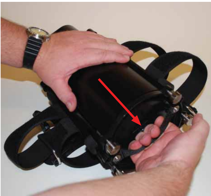
Figure 1-12. Remove the End Plate.
