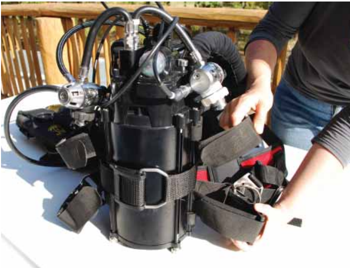
Figure 1-86. Latch the cam band, securing the gas processor to the harness back panel.
